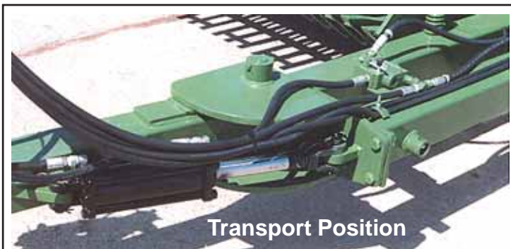
Two 3" x 31" hydraulic cylinders with case hardened shafts provide for bucket dumping action. Hydraulic lines to tractor are included.
