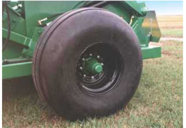
Flotation Tires: 16.5L x 16.1 are standard providing for mobility on soft fields.
