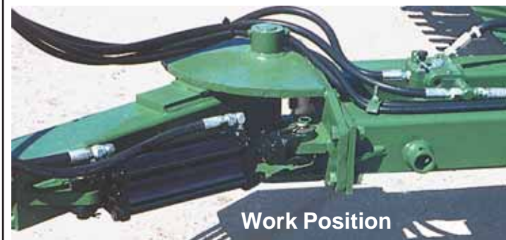
Standard Swing Hitch is hydraulically actuated to position the hitch for either offset work position or transport.
