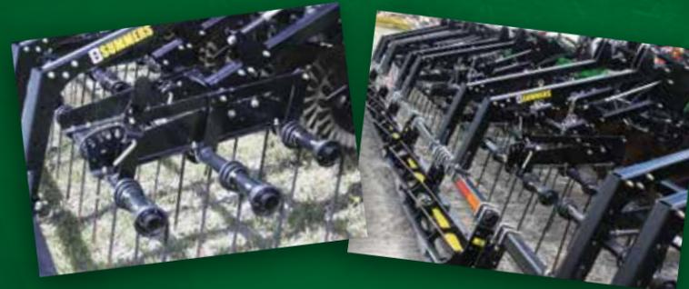
To create the ideal field finish, the VRT Renegade comes standard with an adjustable three-bar harrow and rolling baskets. The rolling baskets feature Summers' patented internal mud scrapers to prevent mud build-up. They also include hydraulic down pressure, which can be adjusted from the cab.
