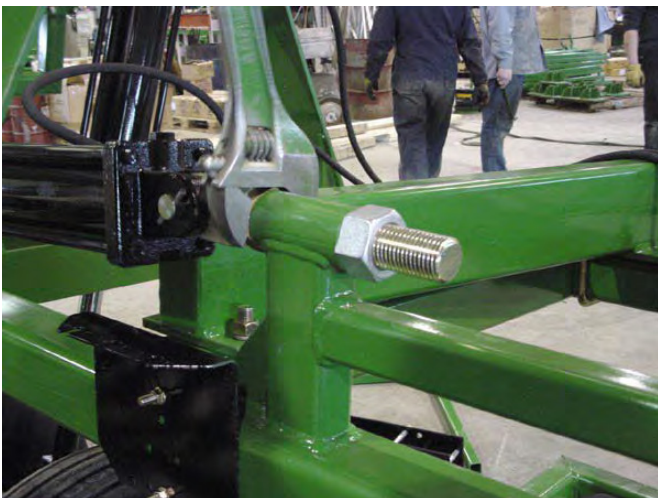
46. Tighten Wing Lift Cylinder eye bolts (above).
