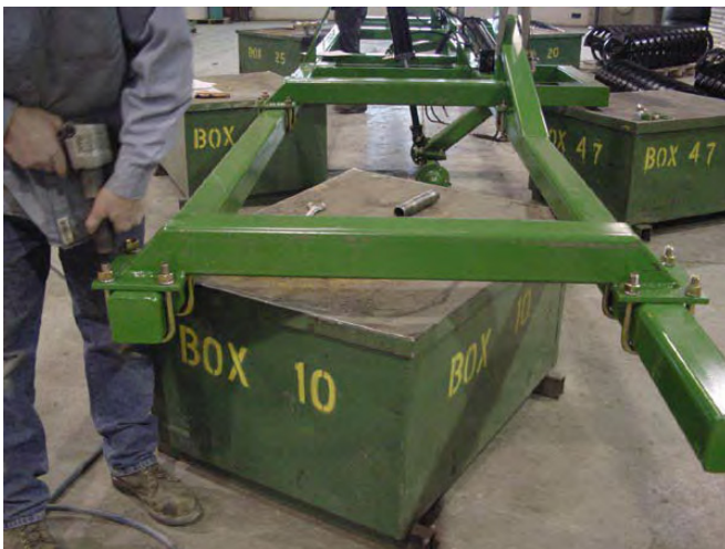
24. Align Wings with Center, tighten u-bolts.
