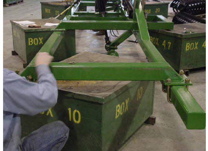
23. Outside Cross Brace.
