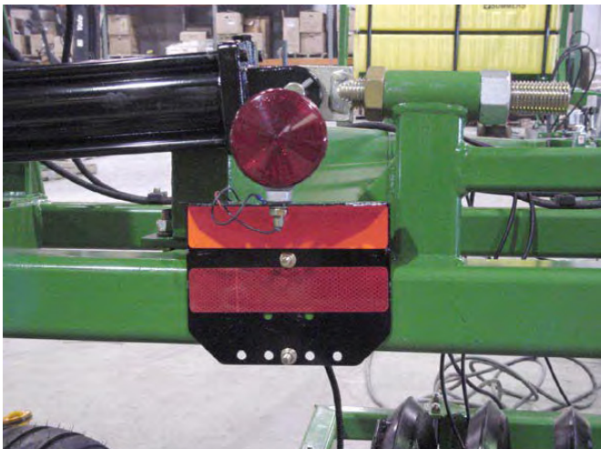
71. Rear Red Light installed.
