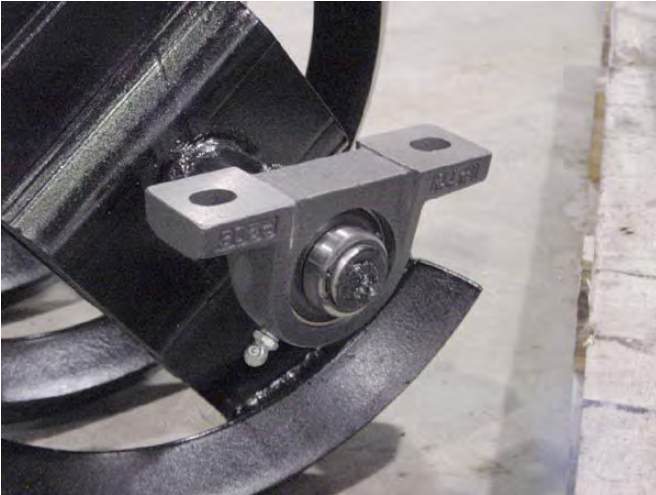
53. Bearing installed with snap ring.
