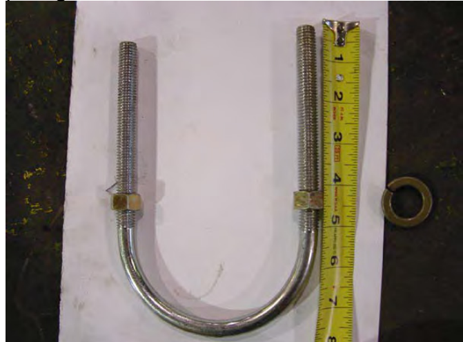
54. Pre-assembly of 1/2" nuts on bearing attach u-bolt.
