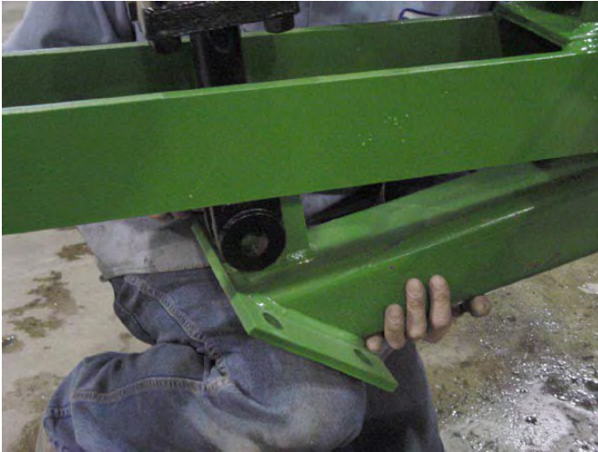
10. Connect rod end of main lift cylinder.
