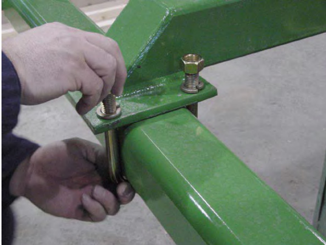
22. Secure Cross Braces.
