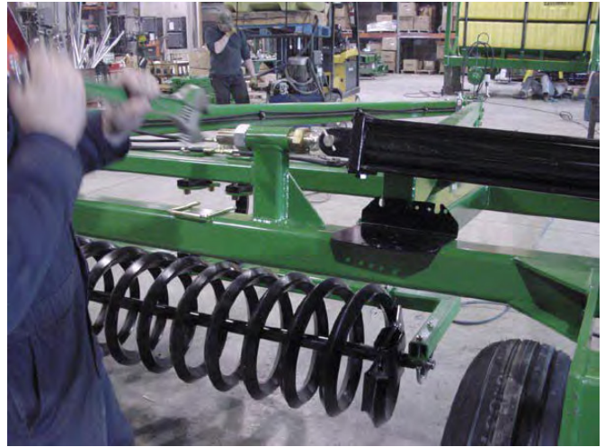
45. Adjust eye bolts so Wing rests on Center.
