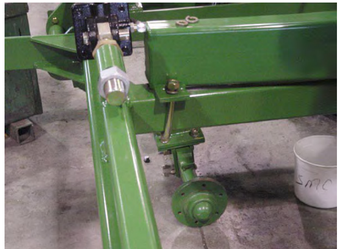
35. Rear u-bolt installed.
