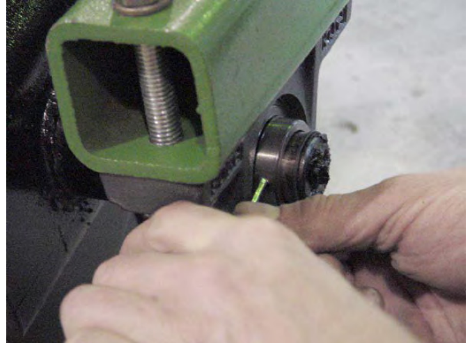
57. Center Coil and tighten set screws in bearings.
