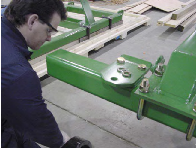
47. Mark frame using layout drawing, located clamps.
