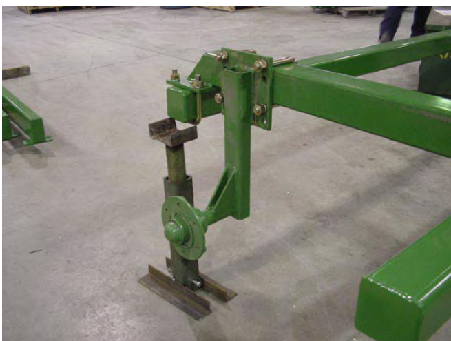
26. Left hand Wing Axle installed.
