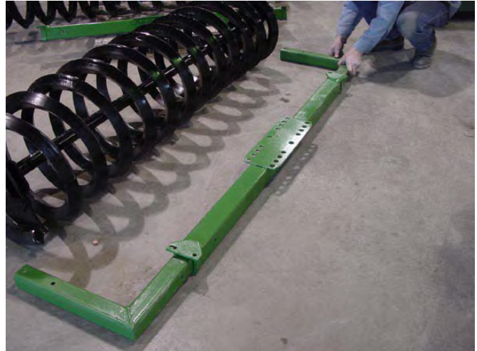
52. Identify Left and Right Hand Coils by comparing to bolt heads.
