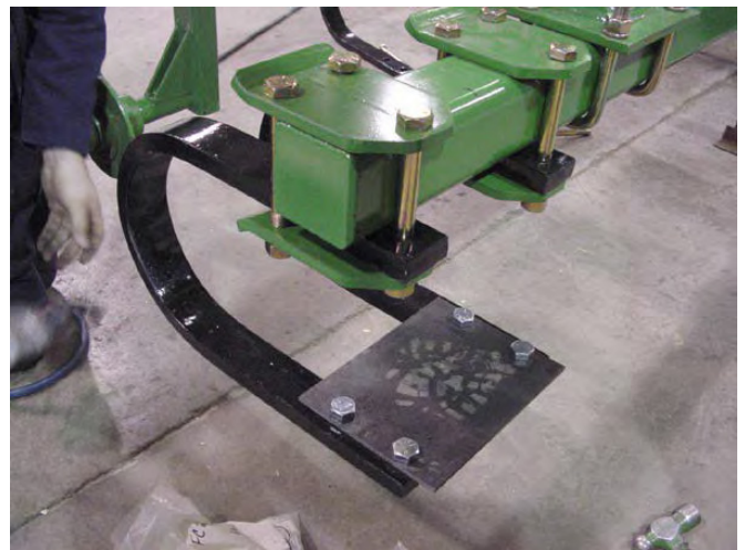
50. Tighten C-Shank mounting hardware.
