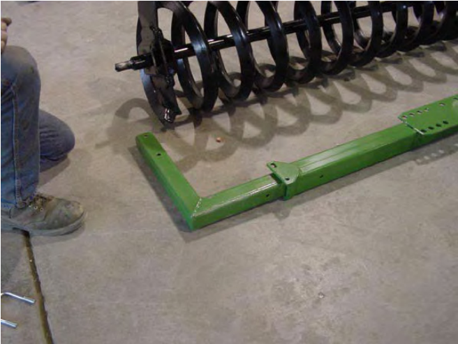
51. Lay out Coils and Pull Frames.
